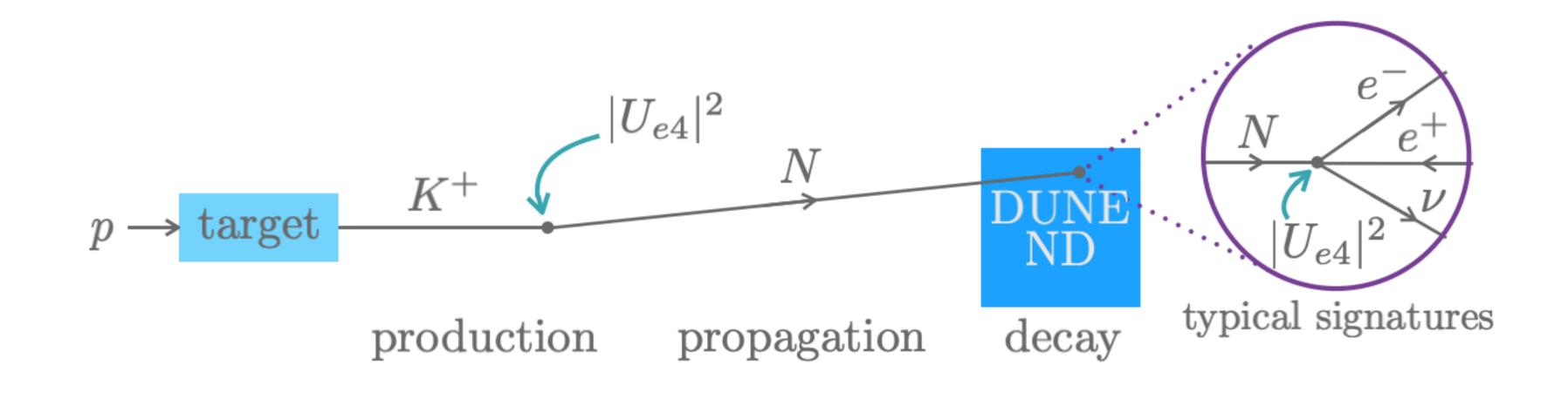
Heavy neutrinos can be produced at beam dump facilities via meson decays and decay in the near detector into leptons and lighter mesons.
