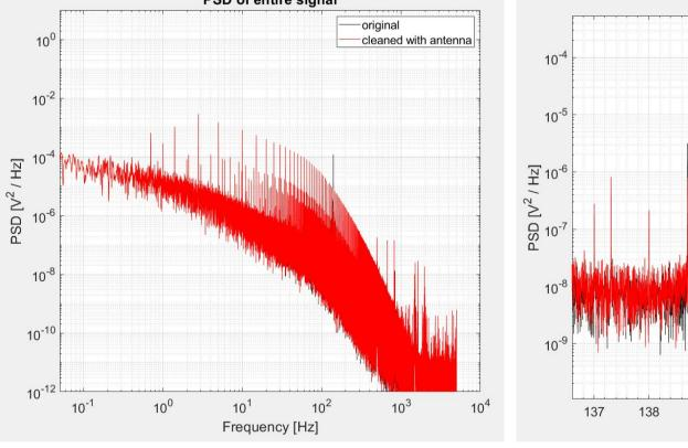
When the 30 Hz LED train data is denoised using ANC, we see that there is a significant reduction in the noise continuum at frequencies below 1 Hz. The noise peaks due to the PTs (1.4 Hz and subsequent harmonics) are also reduced or even completely eliminated.
