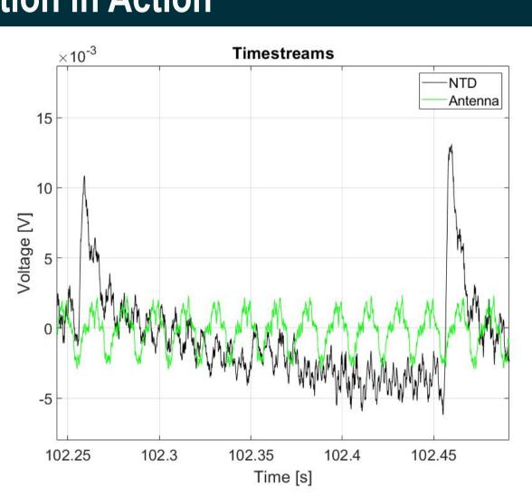
Once the convolution is complete, the resulting signal strongly resembles the electrical noise seen in the data!
