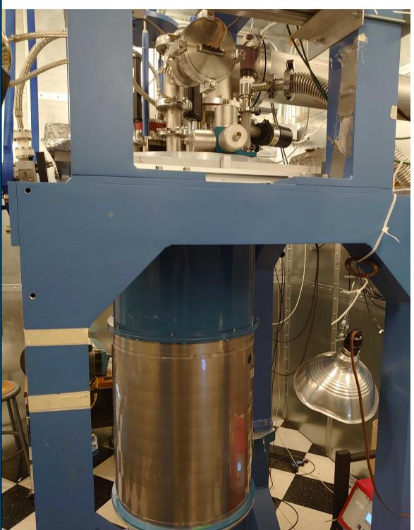
In the lab at UC Berkeley, we have a dilution refrigeration unit (left) in which we can cool our devices to ~ 12 mK. We work with both NTD-Ge calorimeters, which are similar to those used in CUORE, and TES-based light detectors as part of research and development for the CUPID experiment.
