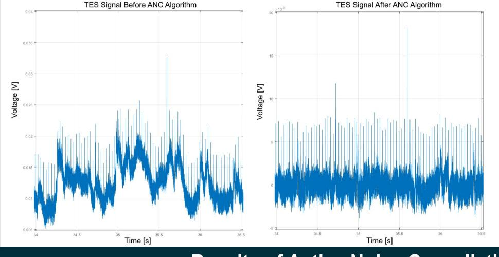
For the ANC algorithm, the convolution happens as the algorithm adapts, rather than at the end of the process as is done in the LNC algorithm.
