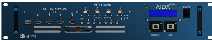
CAD Drawing, 19-inch TLU
