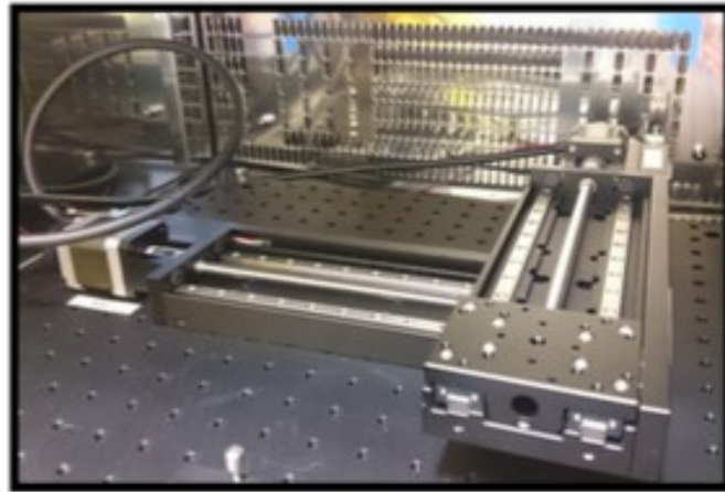
15 cm range translation stages inside the climate chamber SiPM Gain Stability – UB, Prague
