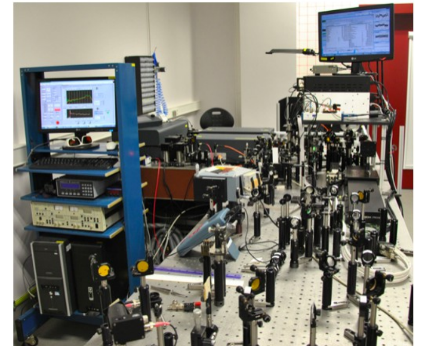
Setup of the pump-and-probe testbench in Vilnius, Lithuania. (Image: AIDA-2020 WP14)
