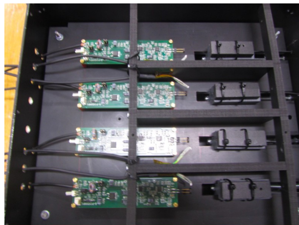
15 cm range translation stages inside the climate chamber SiPM Gain Stability – UB, Prague
