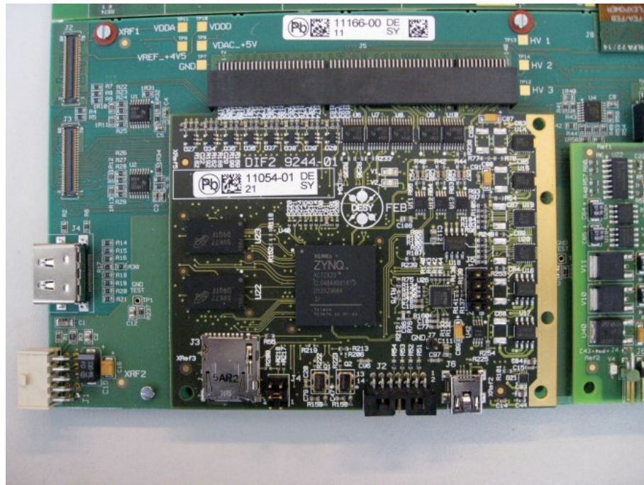
Current detector interface card - SDHCAL
