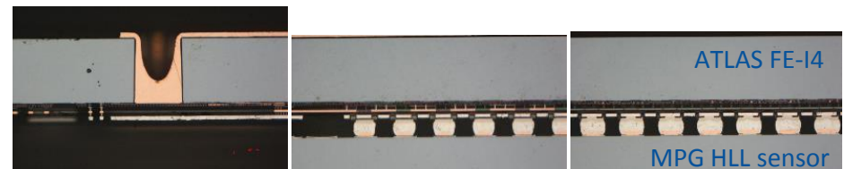
Cross section of module with 80 \mu m thick ATLAS FE-I4 backside TSV ROC
