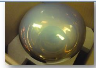
Direct TPB coating on PMT
