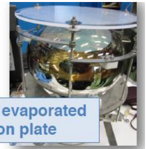
Direct TPB coating on PMT
