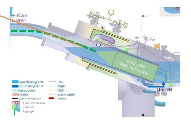
Needed in plane bending of the SC Link before the "descent". Exact geometry to be drawn – including supporting structure fixed to the ceiling
