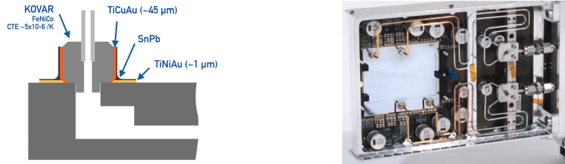
Figure 9: (left) Schematic cross-section of the machined connector welded to a capillary and soldered to a silicon substrate. (right) Picture of the 4 capillaries of the NA62 GTK detector welded to the Kovar connectors which are soldered to the silicon micro-channel cooling plate.
