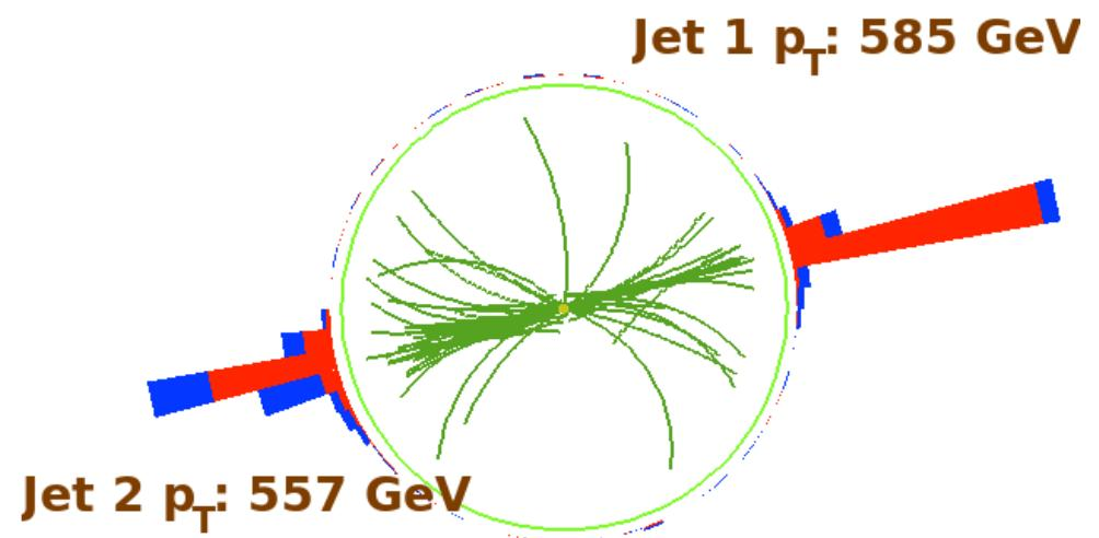
Two jets clustered using anti- $k_T$  algorithm with  $R=0.7$
