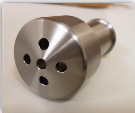
Modified extraction electrode machined and will be tested at Offline-2 and GPS
