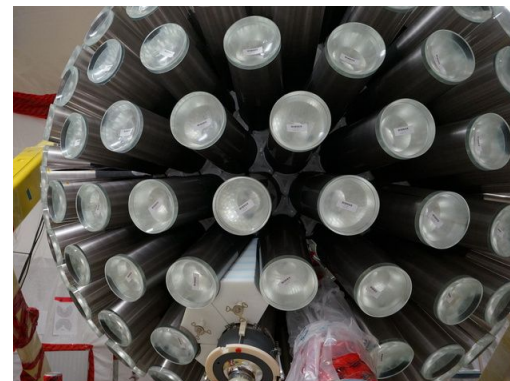
Light guides dressed in reflectors
