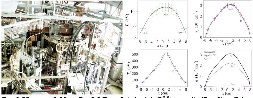
$R_0 = 0.55 \text{ m}, a = 0.08 \text{ m}, B_t = 2.2 \text{ T}, q = 2.1, \hat{s} = 1.1, O^{6-8+} \text{ impurity } (Z_{\text{eff}} = 3), \tau = 7.1$
