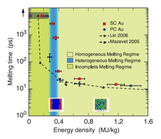
located inside the gray shaded area are beyond the instrument limit of 3 ns for our experiments, and the two data points on the left are from measurements of below damage threshold.
