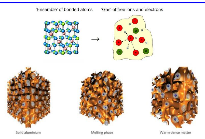
Molecular dynamics simulations of the formation of WDM indicate that the ions (dark blue) abandon their lattice positions. Although core electrons (grey) remain mostly unchanged, the delocalized conduction electrons (represented by orange isosurfaces) are disturbed from the very regular structure in the lattice. (Credit: SLAC National accelerator Laboratory)
