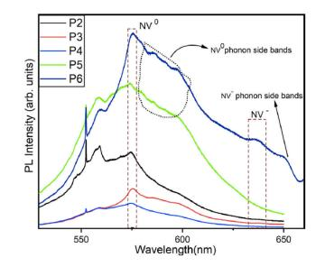
Room temperature PL emission spectra of nitrogen doped films showing the presence of NV0 centres in sample P2–P6 and their phonon side bands. Only sample P6 indicates the presence of NV– centres.
