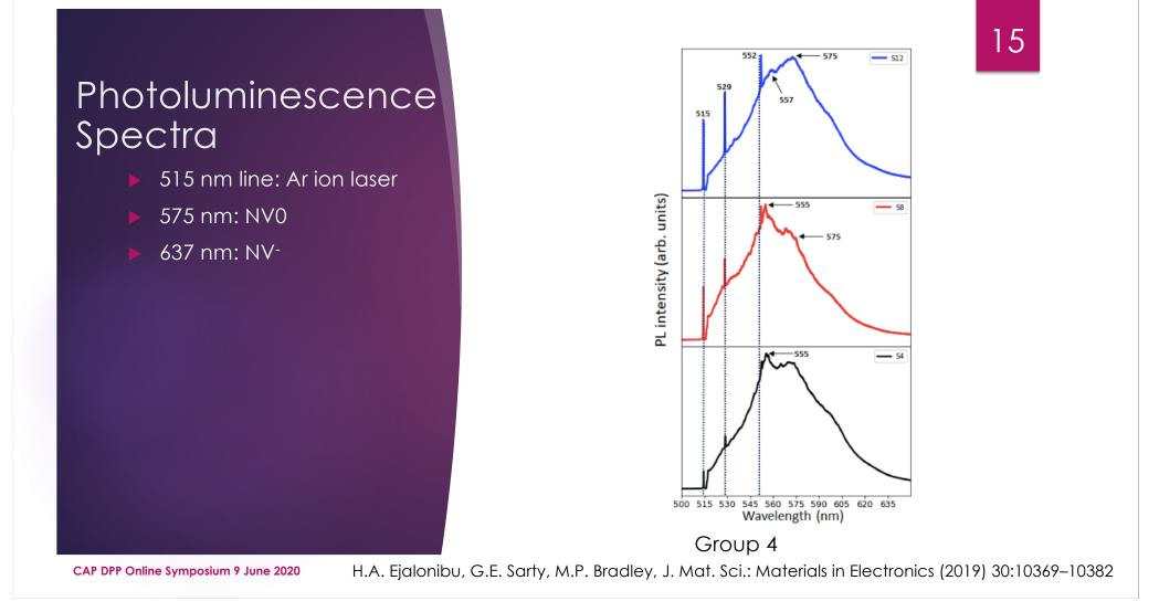
Only sample S9 exhibited a (small) NV<sup>-</sup> 637 nm PL peak S9 growth conditions: 100 -1-10  $H_2$ -CH<sub>4</sub>-N<sub>2</sub> flow (sccm)
