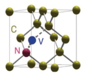
The NV Centre in Diamond- a special type of defect: A substitutional nitrogen (N) *adjacent* to a vacancy (V) Can be made in various ways:
