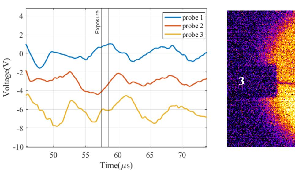
**Figure 8: Processed floating probe signals**
