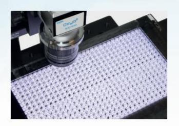
nanoGPS Oxyo® technology is based on taking a picture of a patented patterned substrate, and interpreting this picture into position (x, y) and orientation  $(\theta)$ .
