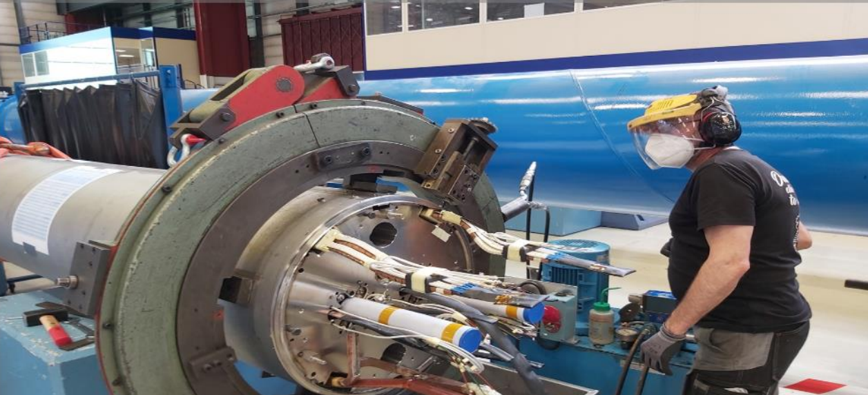
S3 preparing for coil replacement
