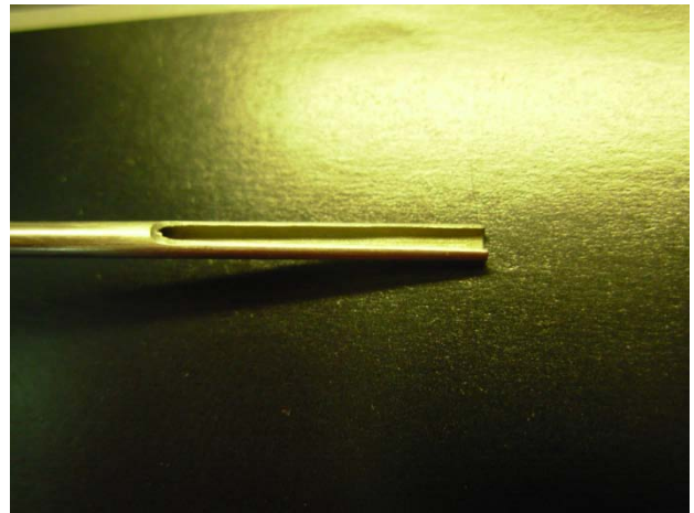
A relative humidity sensing fibre (tip-coated) in its custom produced needle housing
