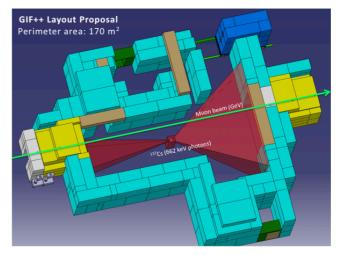
layout permits simultaneous high-rate irradiations of very large-size muon detectors. The facility is expected to be operational in 2011.
