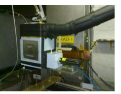
Coldbox for ATLAS SCT structures in lab with water cooling
