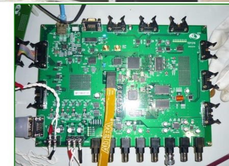
Developed FPGA-CPU board for precise control of magnet PS
