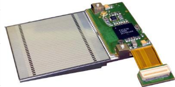
Fig. 5 The analog memory cell of PACE3
