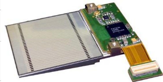
Fig. 5 The analog memory cell of PACE3
