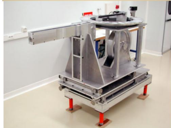
"Carousel" brick dispensing and storage system
