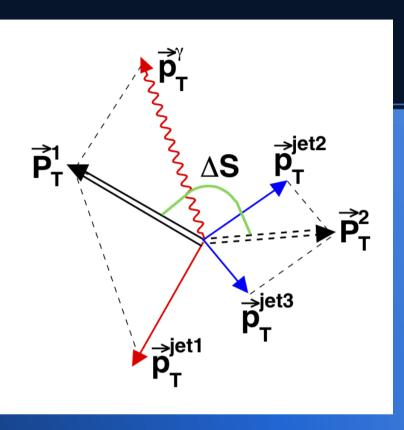
$$p_{T} = \frac{1}{\sqrt{2}} \sqrt{\frac{\vec{p}_{T}(\gamma j_{0})}{p_{T}^{\gamma} + p_{T}^{j_{0}}}} + \frac{\vec{p}_{T}(j_{1}j_{2})}{p_{T}^{j_{1}} + p_{T}^{j_{2}}}$$
