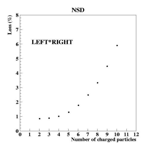
Losses in NSD as a function of number of particles seen in each telescope.
