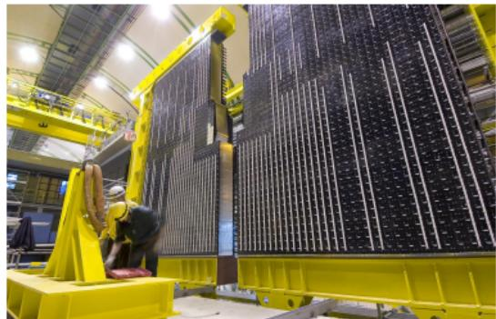
**ECAL:** For  $\gamma$  and  $\pi^0$  detection, and  $e$  identification
