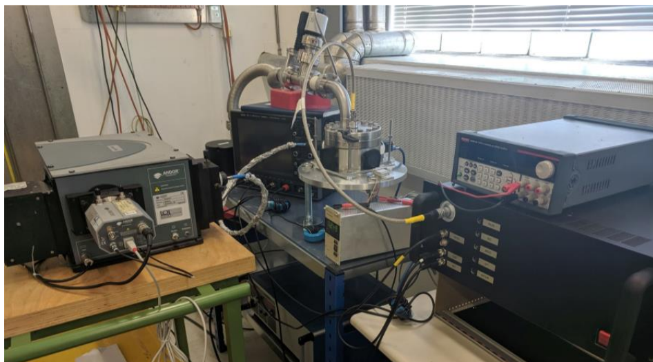
The MARX generator supplies a pulsed voltage up to 10kV and frequency up to 6kHz
