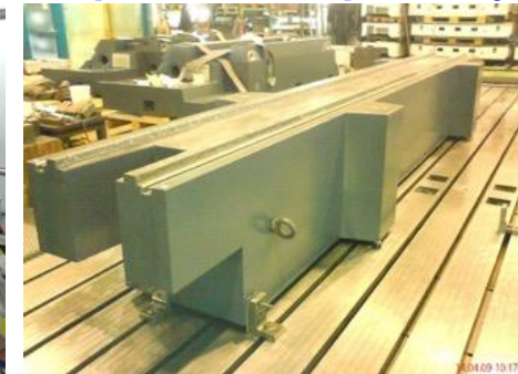
Damping girders with high-frequency absorption capacity
