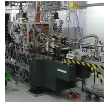
Damping girders with high-frequency absorption capacity
