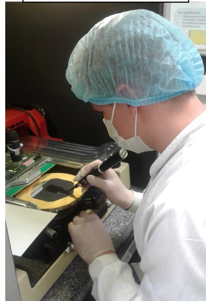
Mounting of silicon prototype modules on HGCAL prototype detector planes
