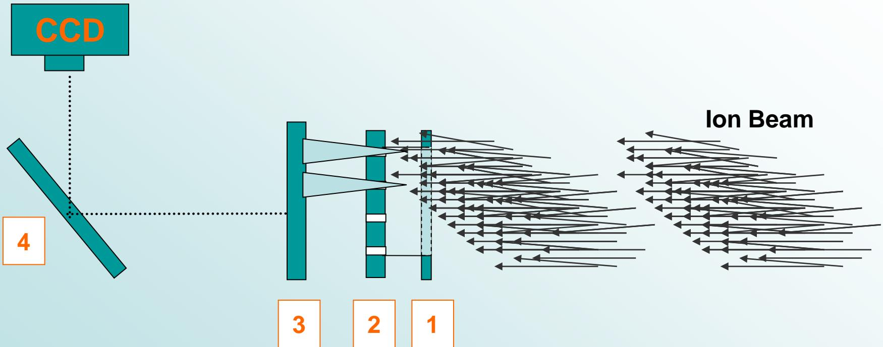
Allow to create an image that portrays the distribution of particles in the beam ( “emittance” )
