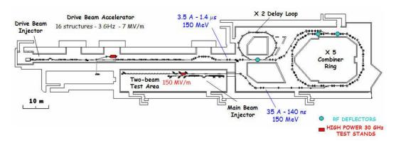
• Test accelerator at CERN to demonstrate the feasibility of CLIC concept.
