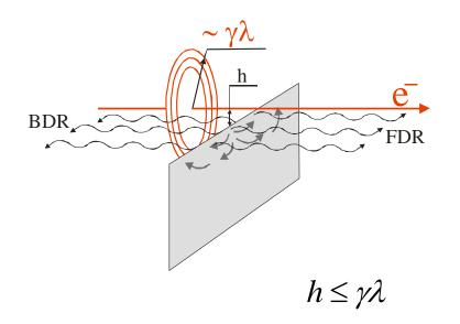
Diffraction radiation appears when a charged particle moves in the vicinity of a medium.
