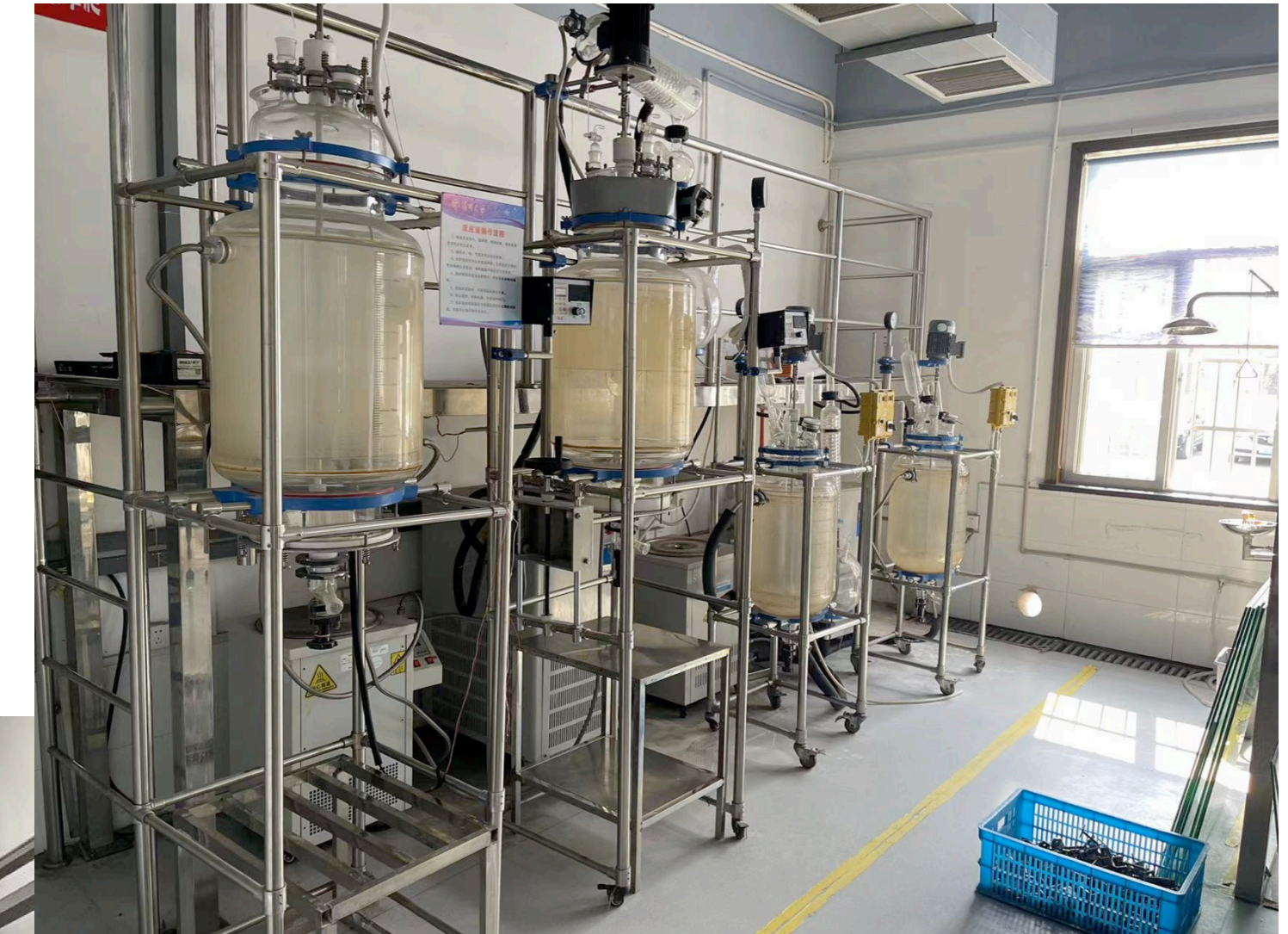
Reaction kettles at YU for the \text{Gd}(\text{MAA})_3 production
