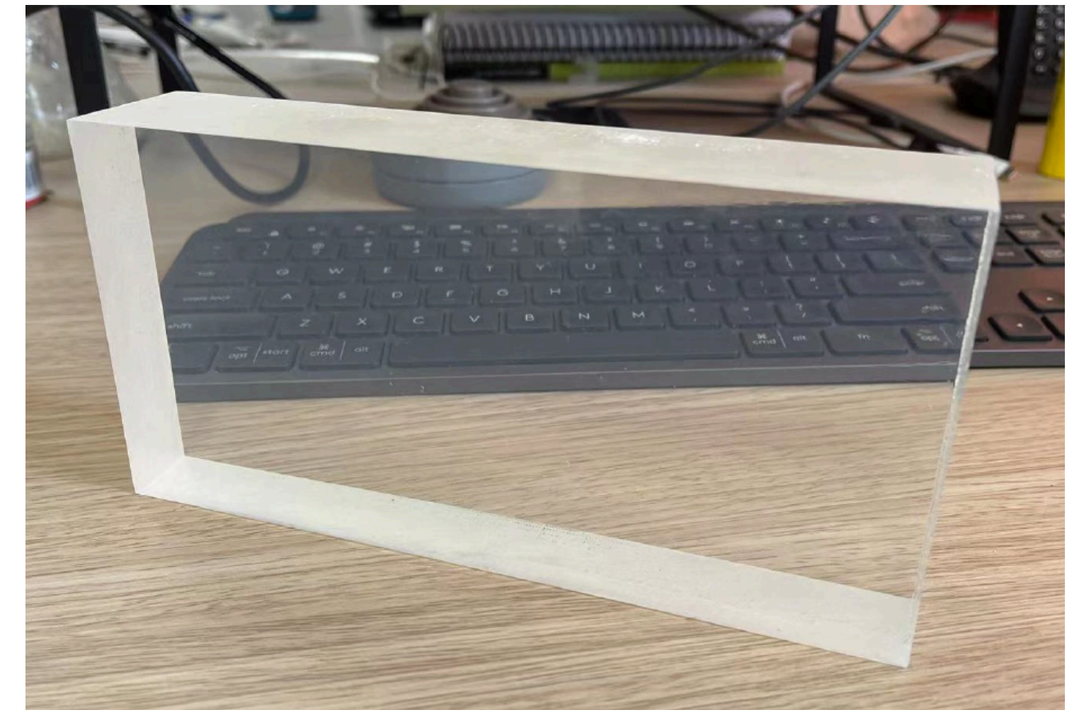
\text{Gd}(\text{MAA})_3 doped acrylic sheet (5 cm thick)
