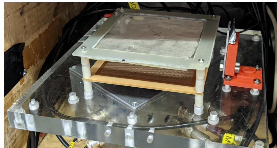
Figure 4: Cross sectional diagram of the MMThGEM structure (top) [2], picture of experimental setup showing the cathode, MMThGEM and 55 Fe source holder (bottom).
