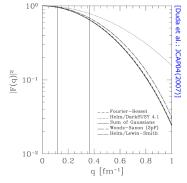
$d\sigma/dT_R \propto F^2(Q^2) \Rightarrow$  suppression of the cross section for large  $Q^2$ !
