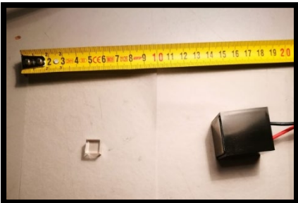
ZnWO_4 crystal = 10 x 10 x 10 mm 3 (detector of reduced dimensions to investigate neutron single-scattering)
