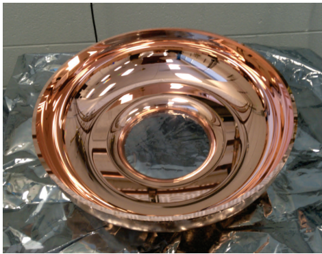
Larry2 - 2 cells precision- machined with mirror finish (rms surface roughness \leq 5 nm)
