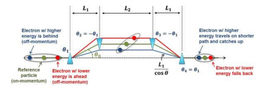
$$\Delta z_2 = \Delta z_1 + R_{56}\delta + T_{566}\delta^2 + O(\delta)^3$$
