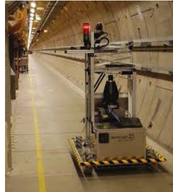
Robot inspecting the XFEL tunnel at DESY
