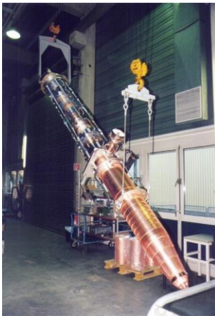
PEP-II 1.2 MW klystron and HVPS
