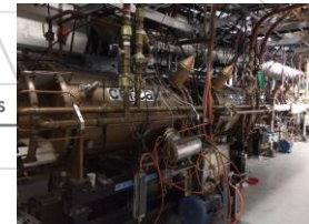
Hadron - 24.5 MHz acceleration cavity
