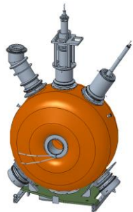
Hadron - 197 MHz bunch compression cavity
