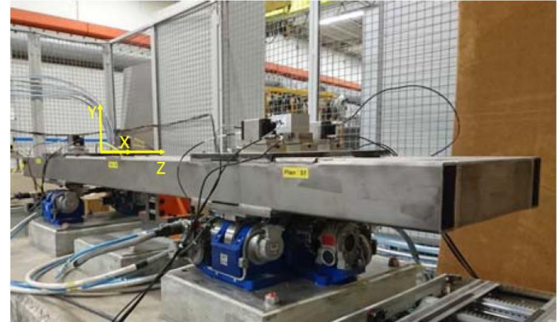
Type 4 MBQ and stabilization system mounted on cam movers (left) and test setup including ZCMs, follower girder and local coordinate system (right).
