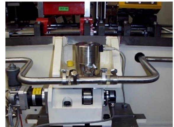
HLS sensor with water pipe connection.
