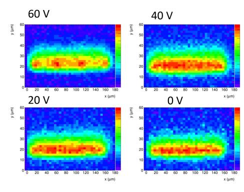
→ no lower efficiency regions between pixels with smaller p-n spacing
