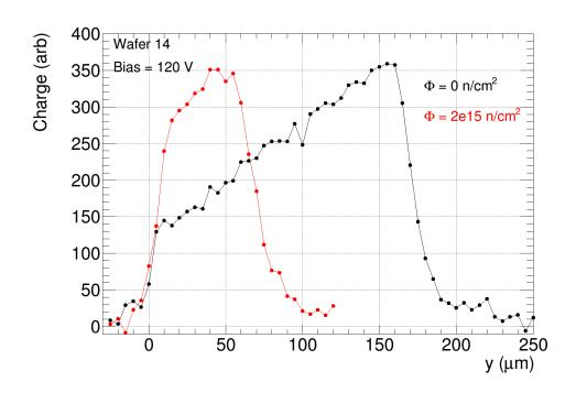
depletion depth shrinks because of irradiation
