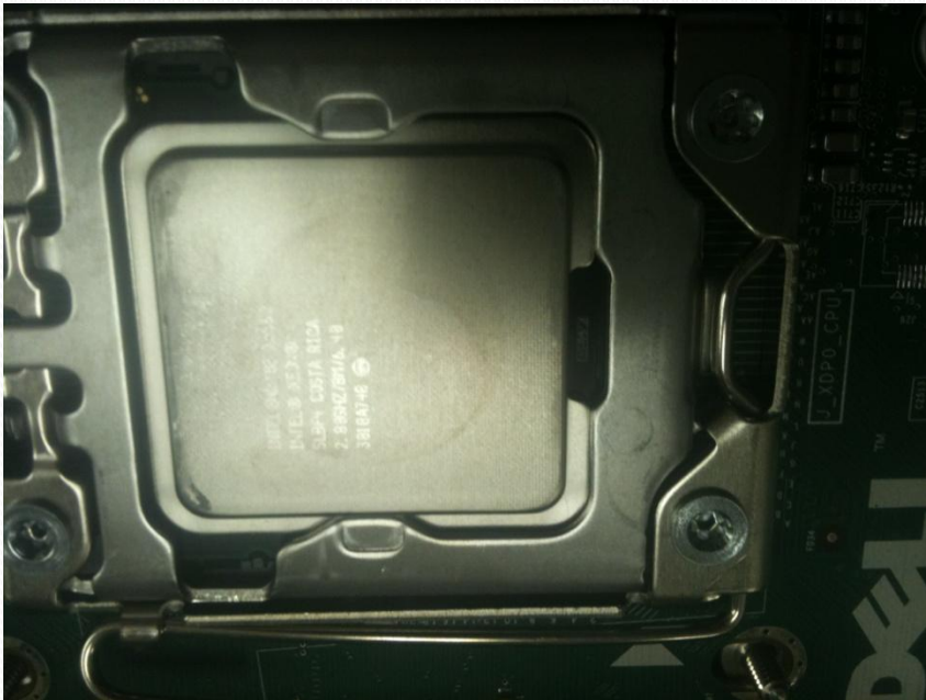
no thermal grease
