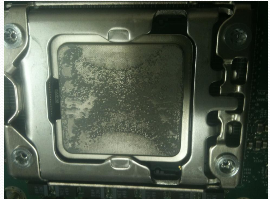
with thermal grease
