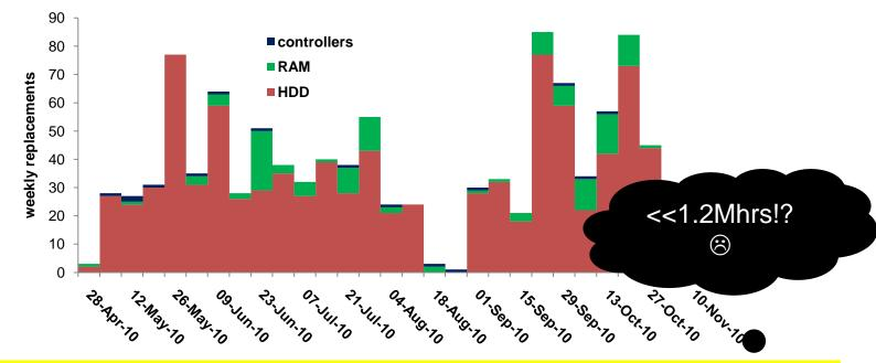
HDD failures/week:30 Hours/week: 168 → hrs/failure: 5.6
