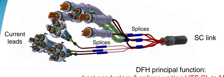
host conductors & splices uniting HTS CL to MgB<sub>2</sub> SC link
