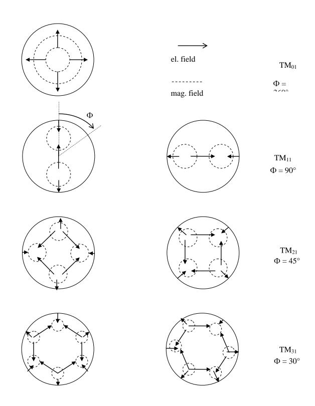
Condition for identical E-field at HOM antenna for dipole and quadrupole mode:  $\sin\Phi = \sin(2\Phi) \Rightarrow \Phi = 60^{\circ}$
