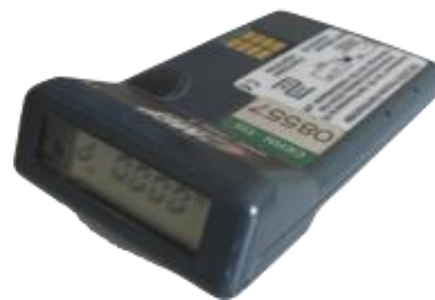
Operational dosimeter DMC: "Operational dose"
