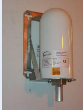
Gas filled, high pressure ionization chamber
