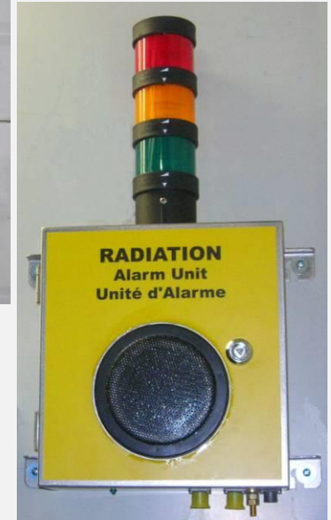
Radiation Alarm Unit (RAMSES)
