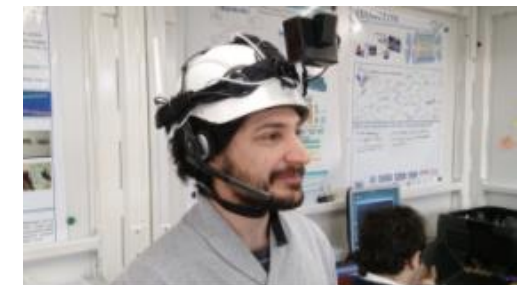
The EDUSAFE integrated safety system uses a camera mounted on the helmet to monitor the working area.
