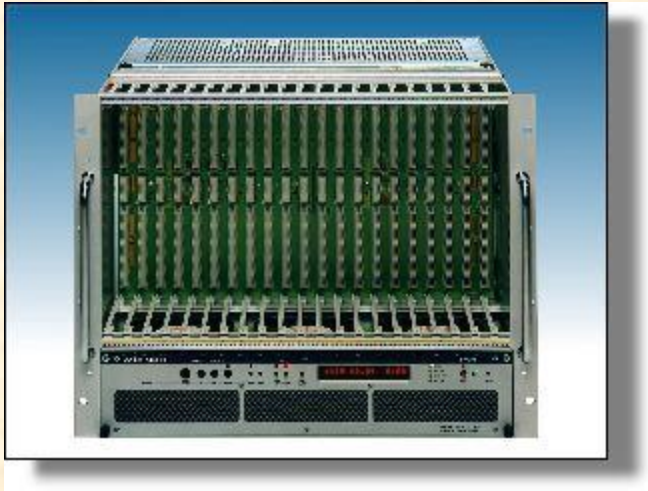
21 slot 6U crate for 19" racks
