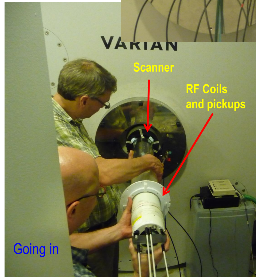
Our “UPenn” PET scanner mounted on the MRI tube
